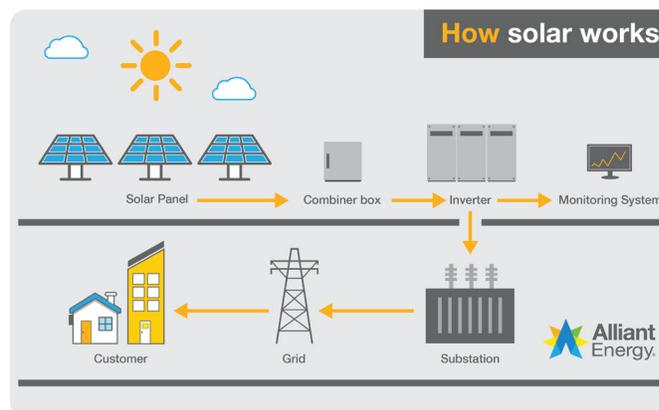
Once the civil sitework is complete, we will begin to install the piles. These metal posts anchor the solar arrays to the ground and support the tracking system that allows the panels to rotate and follow the sun daily from east to west. The graphic above shows the steps it takes to get clean energy from the sun's rays to your home.
